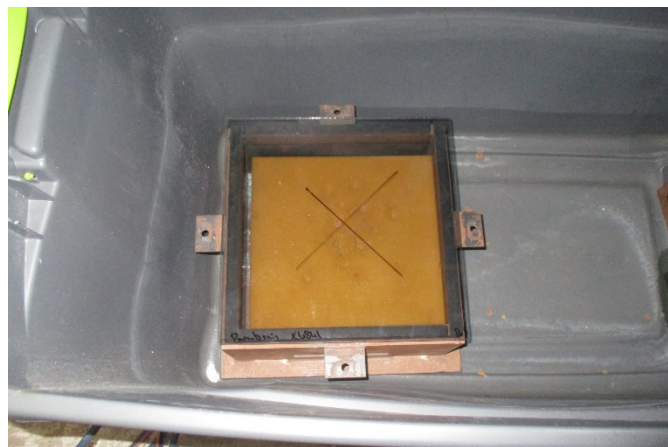
Figure 1: 5.6 Impact, Ball, 3.05m (10ft) Before Impact, Sample 1
