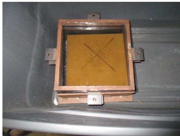
Figure 3: 5.6 Impact, Ball, 3.05m (10ft) After Impact, Sample 1, No Break
