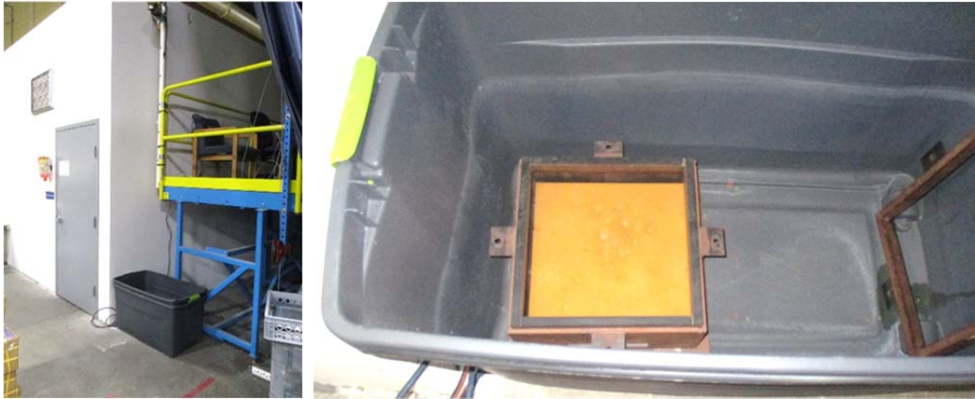
Figure 2: 5.6 Impact, Ball, 3.05m (10ft) Set-up
