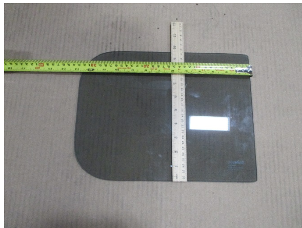
Figure 2: 5.7. Fracture Test Sample before Impact, Sample 1
