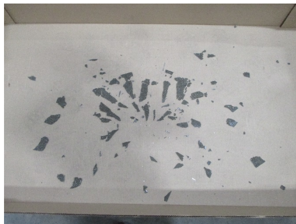
Figure 3: 5.7. Fracture Test after Impact, Sample 1
